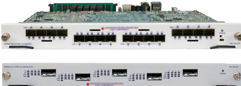
The Spirent fX2 40/10G and 10/1G Ethernet dual-speed test modules deliver the highest density and lowest total cost of ownership in its class. Spirent's Layer 2-3 traffic generation and analysis is combined with powerful network emulation and application traffic to deliver the perfect blend of realism, scalability and performance required to test today's networks.
