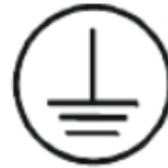
PROTECTIVE GROUNDING CONDUCTOR TERMINAL
