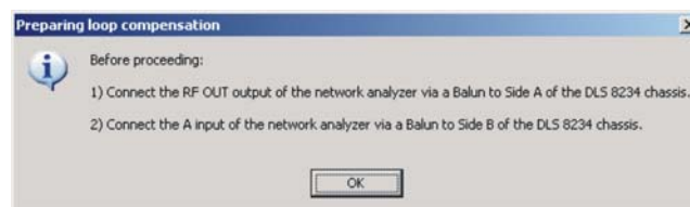
Figure 4-6 Preparing loop compensation instructions
