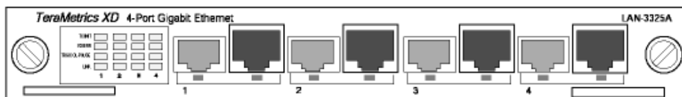
Figure 3-5. Example of LED locations on an Ethernet Dual-media XD Module
