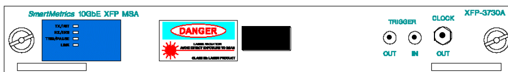
Figure 3-8. Example of LED Location on 10 Gigabit Modules
