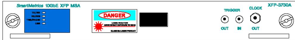
**Figure 3-8.** Example of LED Location on 10 Gigabit Modules
