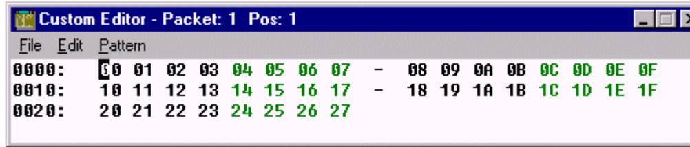
Here you can see that 10 patterns of four bytes each can be edited to form the contents of the VFD. The patterns are shown in alternating colors.
